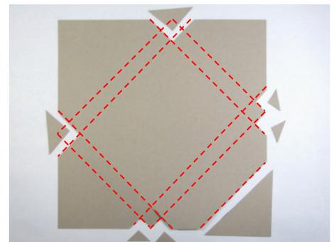
6. Use Paper Snips to cut out the 6 triangular sections shown.
